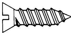
Figure 1 – Thread-forming tapping screw (3.6.10)
