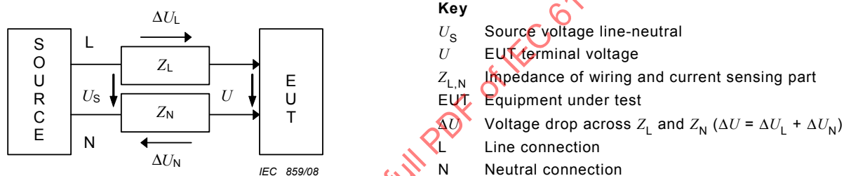
Figure 2 – Measurement set-up for single-phase emission measurement
