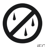
Figure A.1 – Moisture-sensitive symbol (example)
