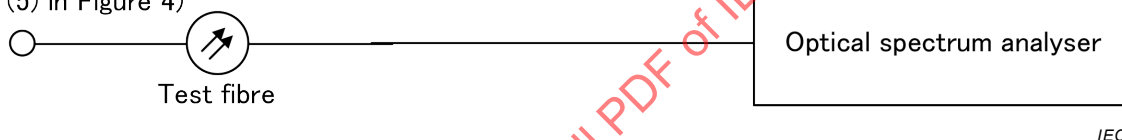
a) Measurement of optical wavelength without WDM coupler
