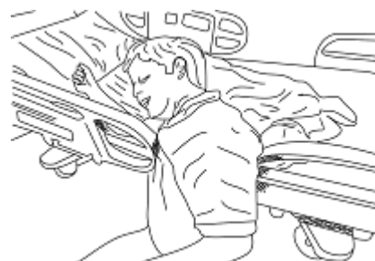
Figure AA.12 – Example of potential PATIENT entrapment in area A below the SIDE RAIL
