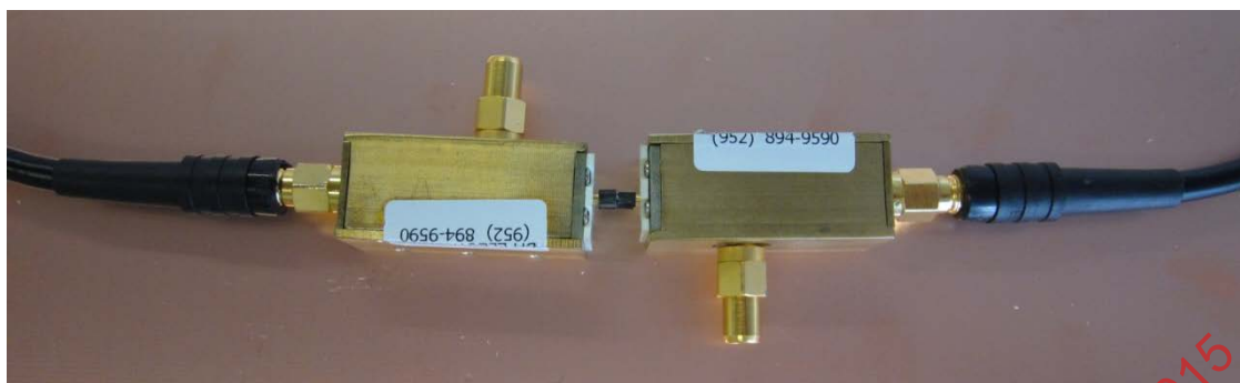
Figure 21 – Back to back balun insertion loss measurement
