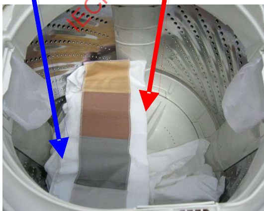
Figure H.11 – Vertical axis washing machine: placement of items in the drum
