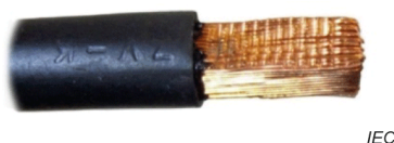
Figure 45 – Large copper single wire end splice (wire end compacted)
