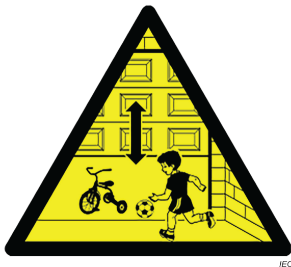
Figure 102 – Example of pictogram warning against child entrapment
