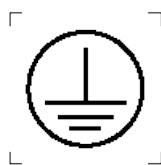
Figure 5 – Symbol IEC 60417-5019: Protective earth
