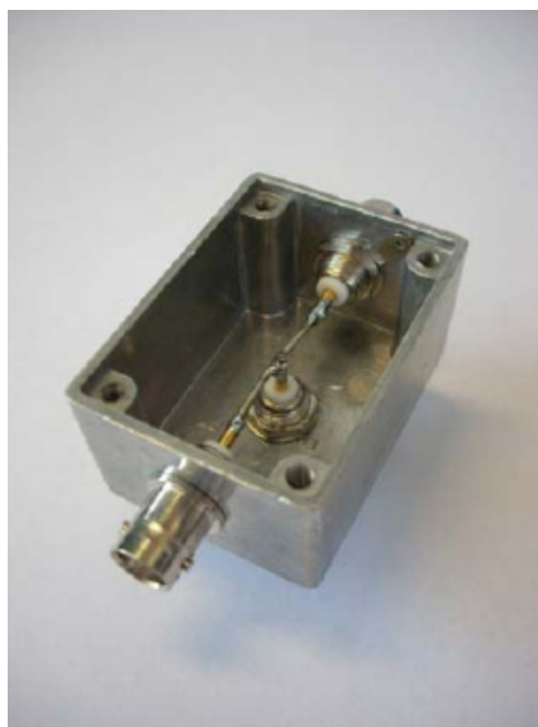
Figure J.3 – Example of construction of a transmitting monopole
