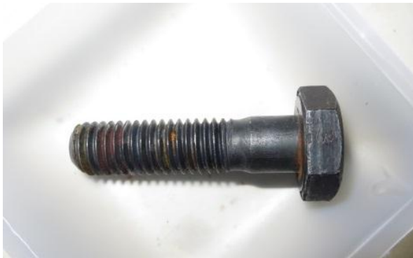
Bolt 3 after deposit removal (0°)
