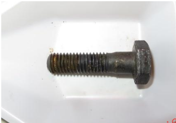
Bolt 2 after deposit removal (0°)
