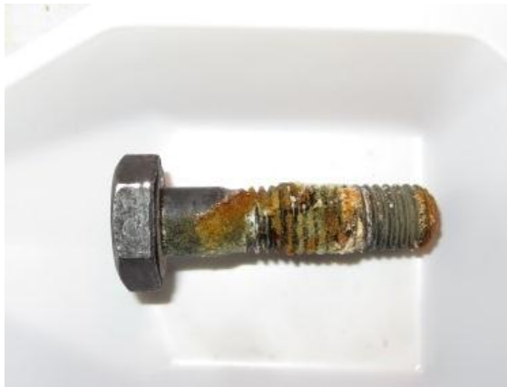
Bolt 2 before removal (0°)
