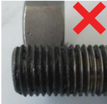
(a) Insufficient Lubrication: Lack of Fill Between Root and Crest of Threads
