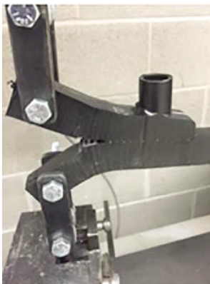
FIG. A2.4 Ductile Failure between Wires-Passing Result
