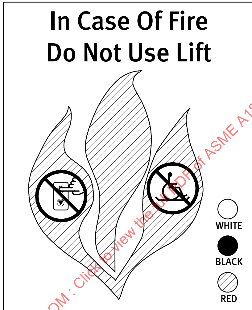
Fig. 2.6.7 Platform Lift Corridor Call Station Pictograph
